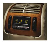
4-zone climate control Individualized comfort can be yours with 4-zone climate control, standard on the \$600 and optional on all other \$-Class models. The system includes rear-cabin controls with a digital display, separate left and right temperature selectors, and automatic blower control.
