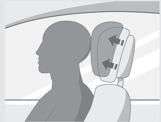
The NECK-PRO head restraints are sensor-controlled.
