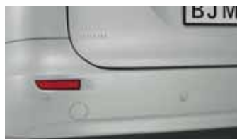
ParkAssist 3 Reverse parking sensor (four-head kit) shown on GLi. Available on all GLi models
