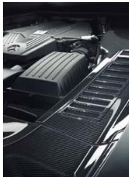
AMG carbon-fibre engine compartment cover
