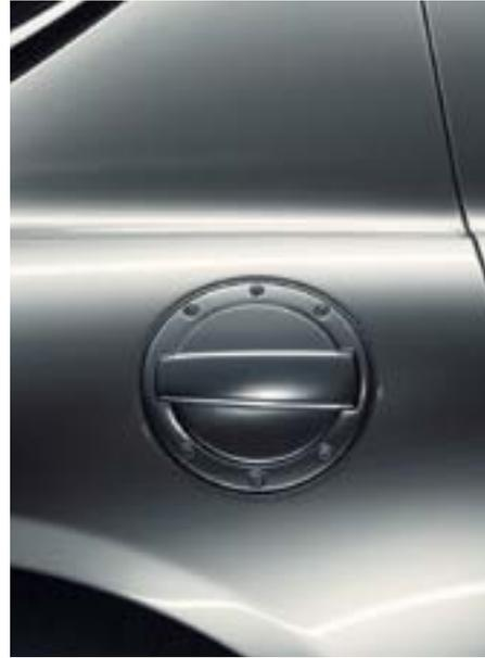
Screw-type solid metal fuel filler cap
