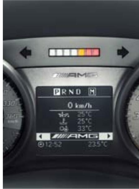
AMG instrument cluster with seven-LED upshift indicator for manual mode
