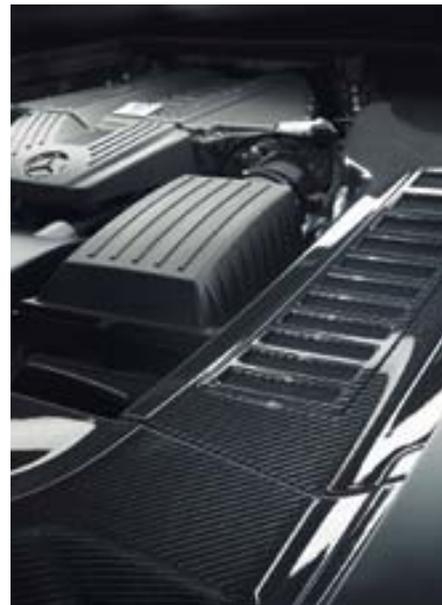
AMG carbon-fibre engine compartment cover
