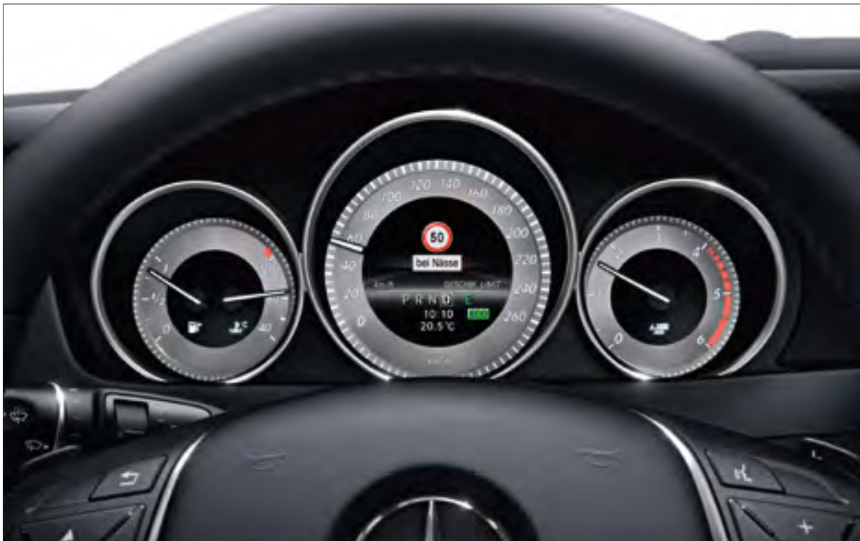
Speed Limit Assist even recognises and displays temporary speed restrictions
