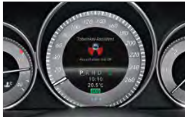
For safer lane changes, Active Blind Spot Assist monitors the hard-to-see areas to the sides of the car's rear
