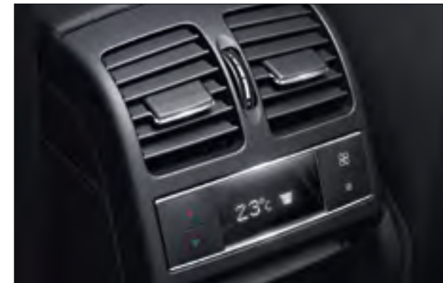
A separate control unit enables those in the rear to set their own temperature settings and blower speed
