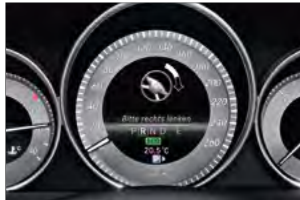
With Advanced Parking Guidance, information on the parking manoeuvre is displayed in the instrument panel
