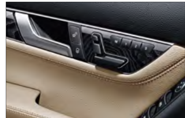
The optional Memory Package allows up to three sets of positions to be stored for the driver's seat, steering column and exterior mirrors
