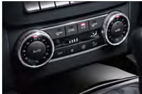
The standard automatic climate control system takes into account sensor data such as inside and outside temperature and humidity
