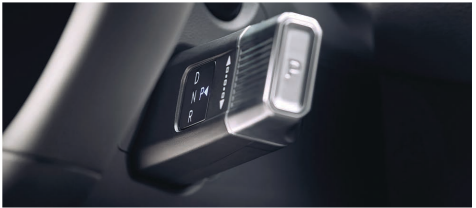
Steering column-mounted Shift-by-Wire gear shifter
