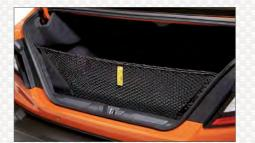
Cargo Net. Neatly holds cargo and prevents it from sliding while the vehicle is in motion.
