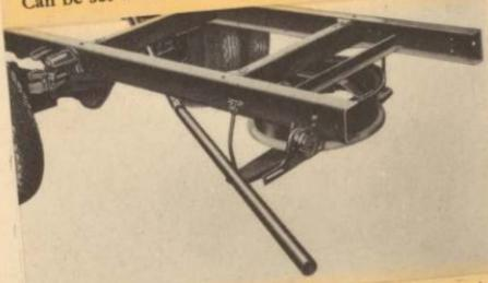
EXTRA LONG EXHAUST PIPE which extends beyond the end of the Ford School Bus frame helps keep injurious exhaust fumes out of the interior of the body.
