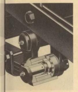
FORESHACKLING of front springs improves steering geometry, makes for easier, steadier, more reliable steering.
