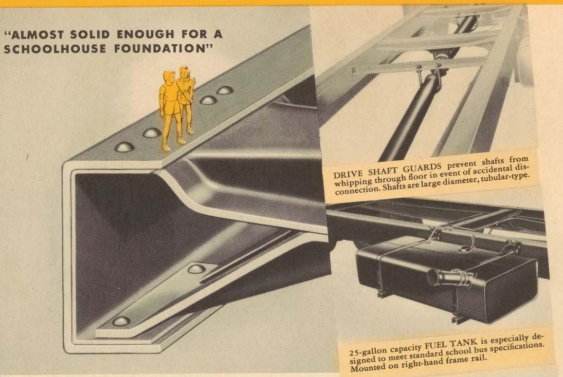
Heavy-duty FRAMES with a depth of 7 in., provide minimum deflection under load, for longer body life. Frame width follows S.A.E. standard of 34 in. Seven strong cross members are rigidly attached to side rails. Cross members in center have massive, flanged, alligator-jaw attachment.
