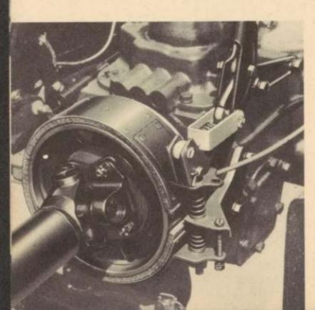
Brake drums feature an effective GROOVE-SEAL designed to keep out dust and water, thereby maintaining brake reliability under varied driving conditions.
