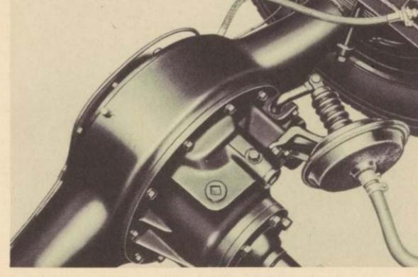
High range of Ford 2-SPEED REAR AXLE on chassis rated at 15,000 lbs. reduces engine revolutions, saves on gas, oil and engine wear. The low range steps up power when extra pulling effort is needed for better acceleration, faster hill climbing ability. A dash button controls the vacuum-actuated shift to either range. Forced flow oiling system gives positive lubrication.
