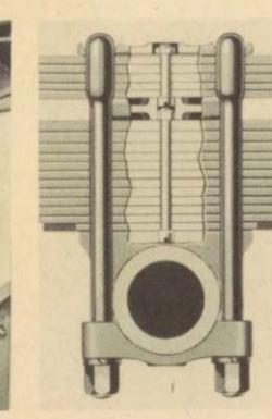
Main and auxiliary springs have INDE-PENDENT CENTER BOLTS. Springs can be serviced separately; bolts last longer.
