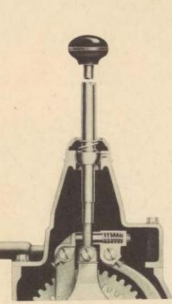
is engineered for endurance. All gears in forward speeds are mounted on antifriction ball or roller bearings to reduce wear. Gears are wide, with strong tooth contours. Sliding shaft and gears are forged from heat-treated alloy steel.
