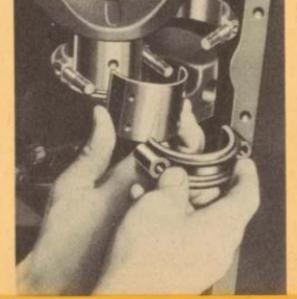
Connecting rod bearings for either Ford V-8 or Six are of easily REMOVABLE type. Oil pan is dropped, bearing cap is removed, bearings slip in.
