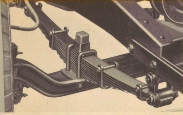
36-in., 11-leaf FRONT SPRINGS have leaves graduated in length and thickness for comfortable riding with varying loads. Springs have wear-resisting, steel-backed, bronze-bushed eyes and hardened steel shackle pins.
