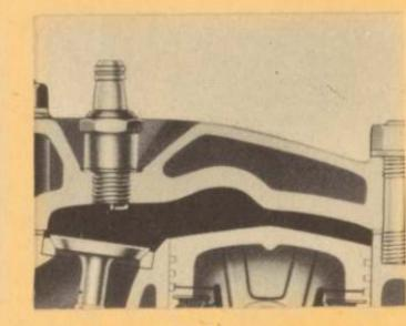
Combustion CHAMBERS are turbocontoured to create high turbulence, promote efficient combustion.
