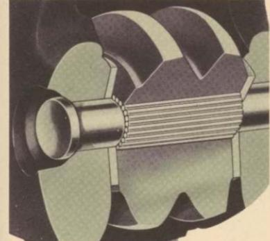
An important Ford contribution to School Bus safety is the NEEDLE BEARING mounting of the steering roller. The needle bearings reduce friction, make steering easier, permit effortless and, therefore, safer driving control.
