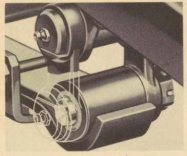
SAFETY-WRAP design of front springs is a notable bus feature. End of No. 2 spring leaf is formed partially around spring eye to assist main leaf, and give double protection.
