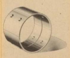
V-8, connecting rod bearings are of "floating" type. With this type of design, both sides of the shell act as a bearing.
