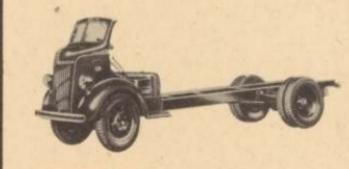
The 134-in. and 158-in. wheelbase C.O.E. models offer cowl to rear axle dimensions of 137 in. and 161 in. respectively, and bring to school bus work such recognized C.O.E. advantages as shorter over-all length, better weight distribution, easier handling, etc.
