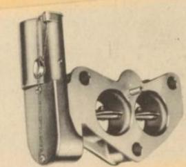
GOVERNOR is optional at extra cost to control road speed, guard against excessive engine speed. Can be set within a range of 1200 to 3000 r.p.m.
