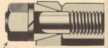
Wedge-type STUD ADAPTERS minimize shearing of rear axle hub studs, by eliminating "play" between stud and flange hole; distribute load evenly to all driving studs.
