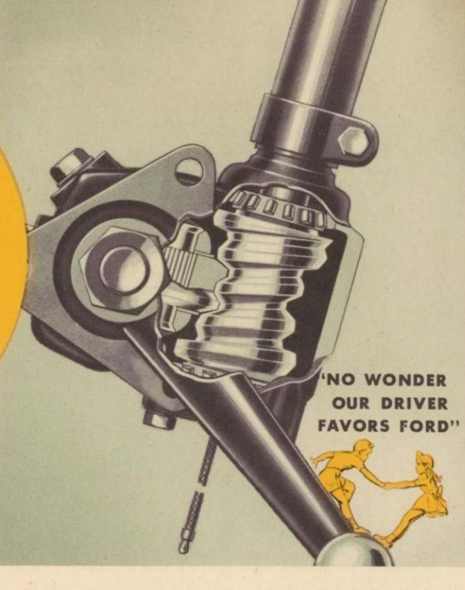
Ford STEERING GEAR works on principle of rolling-action rather than sliding-action, thus reducing friction. Steering worm is supported in two opposed tapered roller bearings which take thrust in either direction. Sector shaft turns in bronze bushings. Both worm and sector shaft are adjustable. (Below) Front axle is rugged, heat-treated alloy steel. Spindles and spindle bolts are extra large for greater safety.
