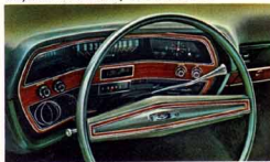
New Flight-Cockpit Instrument Panel puts major controls directly before the driver
