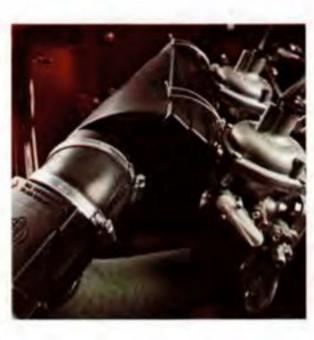
Fuel is supplied through twin horizontal carburetors adjusted and sealed at the factory for Volvo's "dual-induction" emission control. Induction air is thermostatically controlled to a constant temperature by a preheating system in line with the air cleaner.
