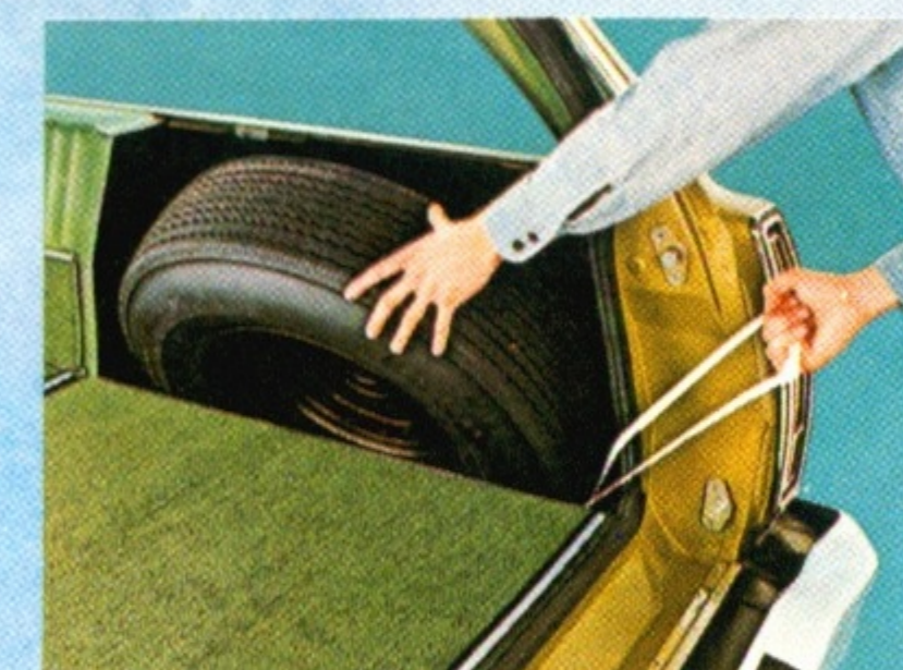
Spare Tire Extractor. Standard on all Ford wagons. With practically an effortless pull the tire is raised onto the load floor from the side well for easy handling.
