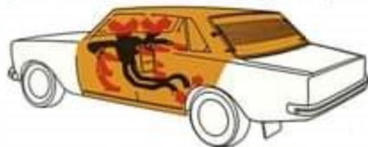
The heating/ventilation/air conditioning system has ten outlets: Two below the windshield, four adjustable monitors on the dash, two outlets for the front doors, two for the rear floor.
