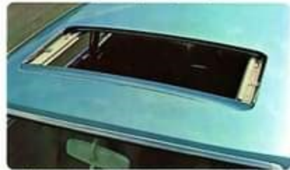
A sliding steel sunroof is optional at extra cost. Completely open, it fits in 14.8" x 30.6" of sunlight. Closed, it fits flush with rest of the roof.
