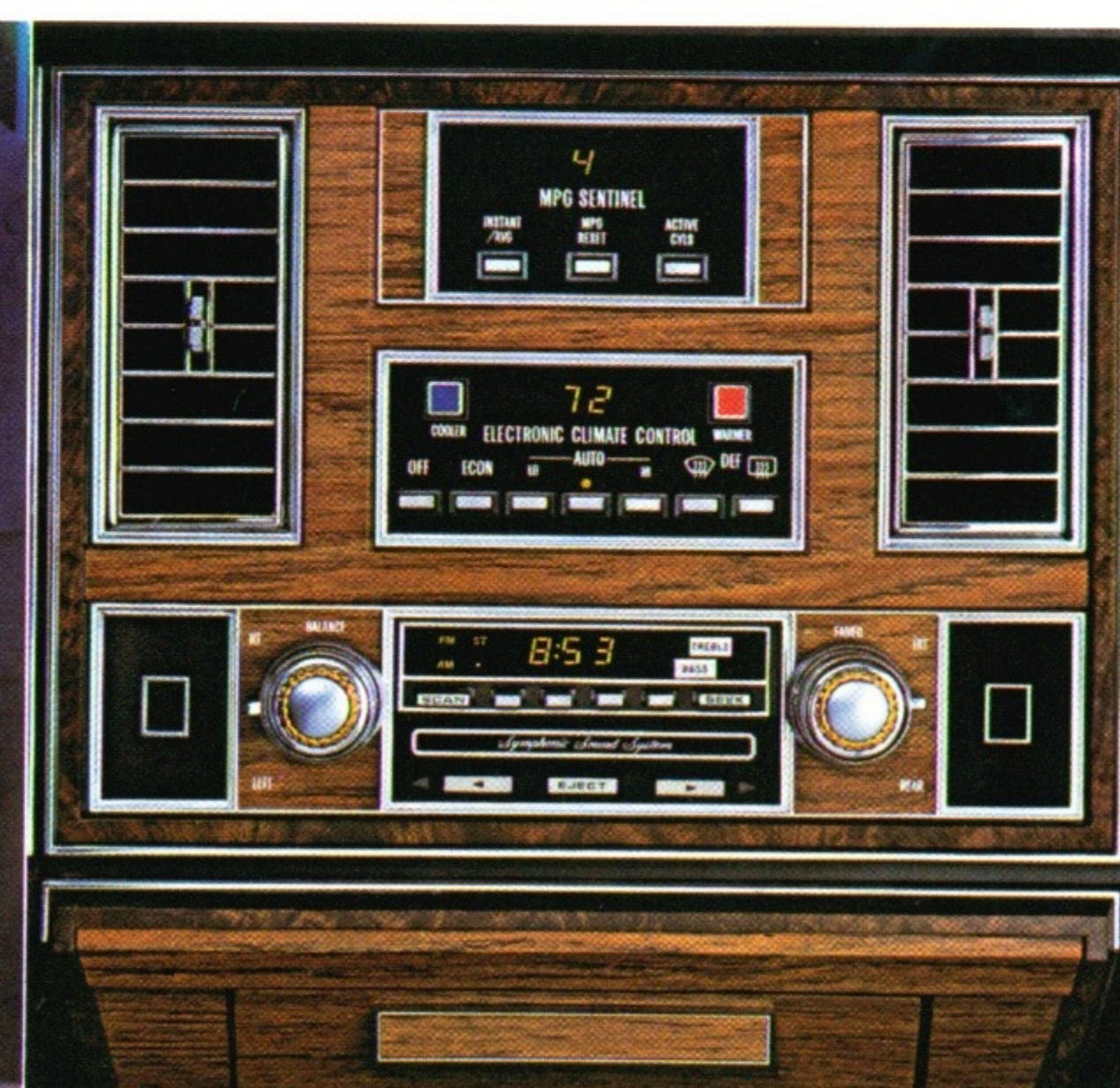
Econominder shows number of active cylinders. (With V8-6-4 engine only.)
