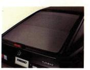
The standard rear window electric defroster clears the view quickly.
