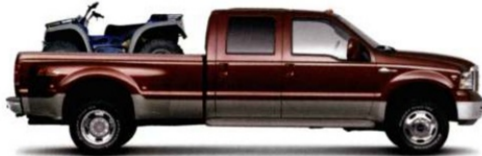
CREW CAB: MAX. PAYLOAD F-350 SRW – Max. 4300 lbs. F-350 DRW – Max. 5800 lbs.
