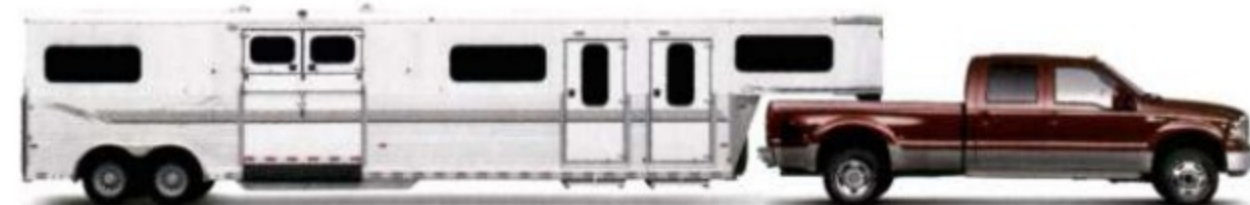
CREW CAB: MAX. CONVENTIONAL/MAX. 5TH-WHEEL TOWING F-250/F-350 SRW – 12,500/16,400 lbs. F-350 DRW – 15,000/16,100 lbs.
