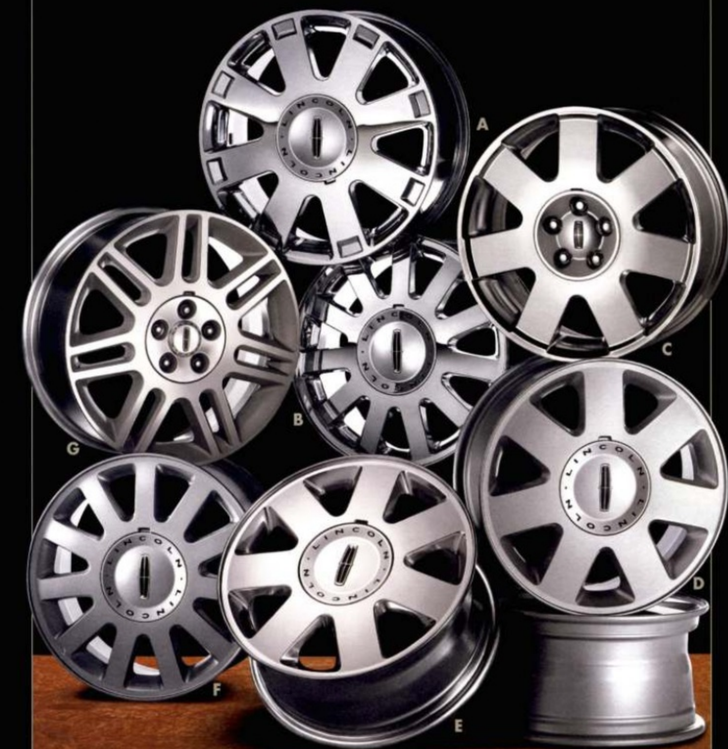
A 17" 8-spoke chromed-aluminum Standard on V-8 Ultimate B 16" 11-spoke chromed-aluminum Available on V-6 Premium C 17" 7-spoke chromed-aluminum Standard on LSE Appearance Package D 16" 7-spoke painted aluminum Standard on V-6 Luxury E 16" 7-spoke polished-aluminum Standard on V-6 Appearance Package F 16" 11-spoke painted aluminum Standard on V-6 Premium G 17" 7-spoke machined-aluminum Standard on V-8 Sport
