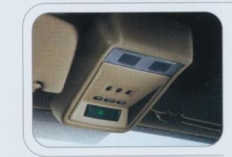
Overhead Console Standard on the LS series, this versatile feature includes a digital compass, dome/map lights, and the HomeLink® Universal Transceiver to activate your garage door opener plus 2 additional home-based units.
