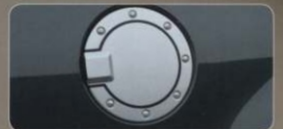
Custom Fuel Door Unique styling complements Explorer's sporty good looks. Made of corrosion-resistant, forged aluminum with a bright satin finish.
