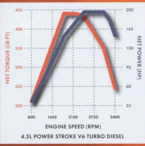
Fire up the all-new 4.5L Power Stroke® V6 Turbo Diesel beast and there're 200 hp and 440 lb.-ft. of torque at your disposal. That's a strong start for any business – best in its class.\* Standard on every Ford LCF, this durable engine is combined with our robust TorqShift™ transmission – the same proven 5-speed automatic featured in many other Built Ford Tough trucks – to deliver maximum power, reliability and efficiency.
