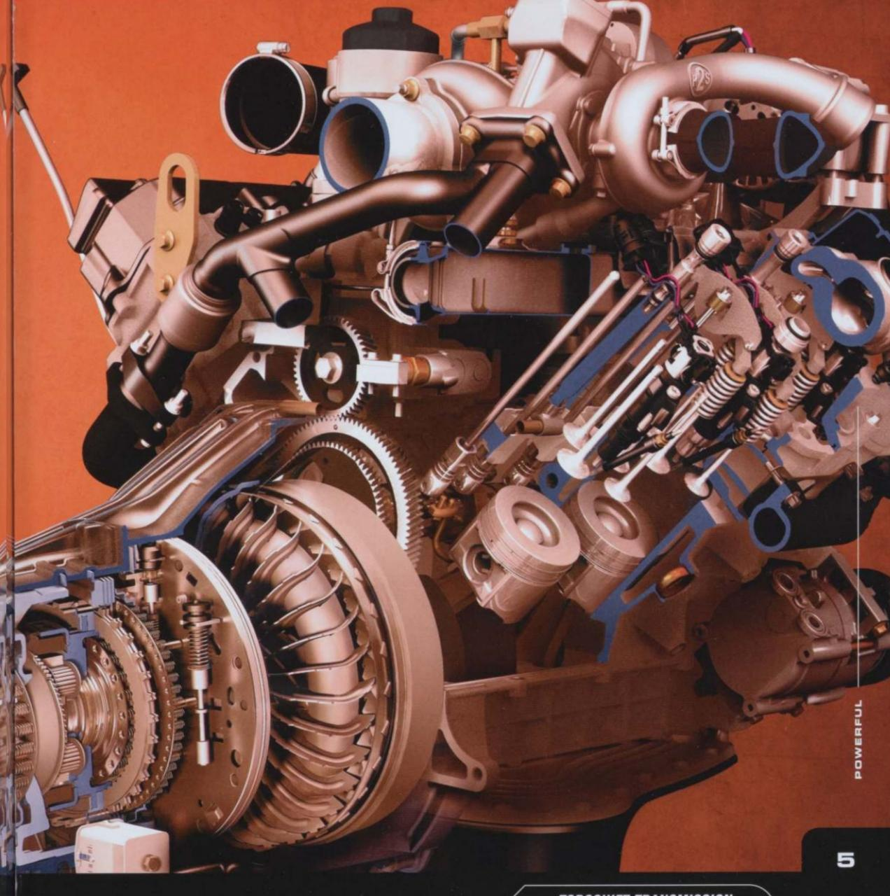
Standard on every Ford LCF, the proven TorqShift 5-speed automatic transmission features pure
