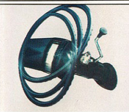
Comfortilt steering wheel adjusts to six different positions for driver's comfort.
