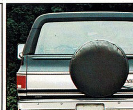
Available swing-out spare tire carrier mounts on the tailgate, provides for more load space inside. Dealer-installed accessory.
