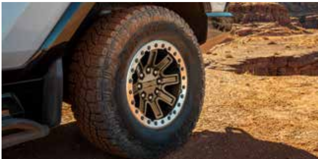
18X9" MULTI-SPOKE BEADLOCK-CAPABLE WHEELS 2 IN GRAZEN METALLIC WITH TECH BRONZE TRIM RING
