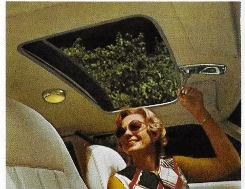
Manually-operated sun roof.
