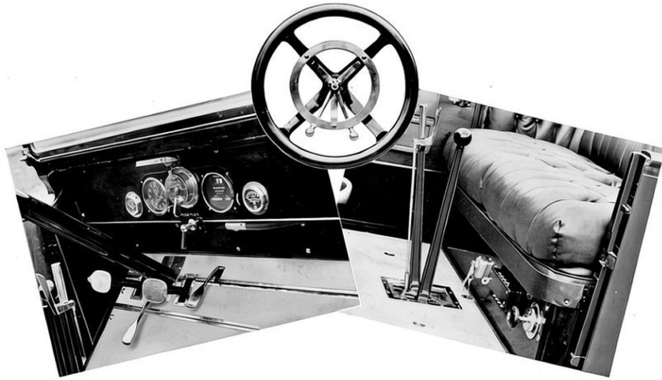
Dash Arrangement, Steering Wheel, Lighting Switch, Hand Air Pump and Muffer Cut-out Lever
