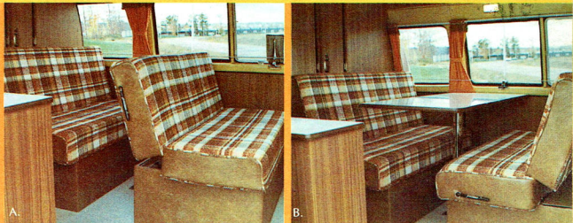
A. Dinette in travel position. Converts to double bed. B. Dinette in dining or card playing position.
