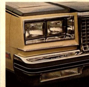
Tungsten-halogen high beam headlight.
