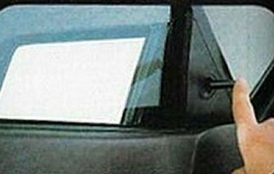
Remote Control Mirrors. Exterior mirrors can be conveniently adjusted from inside car with simple, finger-tip control. Left and right hand available for SL models and left hand only required for SLX models.
