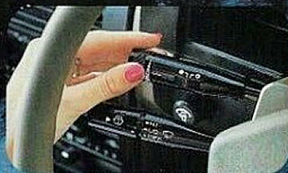
Cruise Control. Graduated easy-to-read speed set dial to enable cruising speed to be pre-set. Does not require speed re-set after every stop. Steering column mounted.
