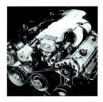
They don't get any bigger than this GTA's 5.T.I.I.O. V8 with tuned-port fuel injection and 240 hp is the largest V8 available in a series-production passenger car.
