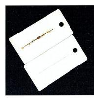
After an equivalent three years of corrosion exposure, the 2-sided zinc-galvanized steel plate, below, shows virtually no corrosion in comparison to the ordinary body steel plate, above.
