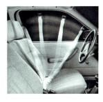
LeMans has automatic safety belts for front-seat passengers. They wrap over your body when you sit down and close the door, Open the door, and they'll whisk away.
