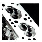
The heartshaped combustion chamber inside the 140 hp 3.11. Vo engine swirts its incoming fuellair mixture for a quick, clean burn, which means more power to you. Under Sunbird's clear outer coat are four more layers of protection: the car color; surfacer/sealer; another layer of primer, and electrically-charged phosphate primer coat.
