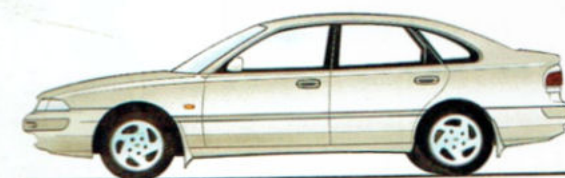
TX-5 Ghia 2.5 litre V6 DOHC EFI with 4WS
