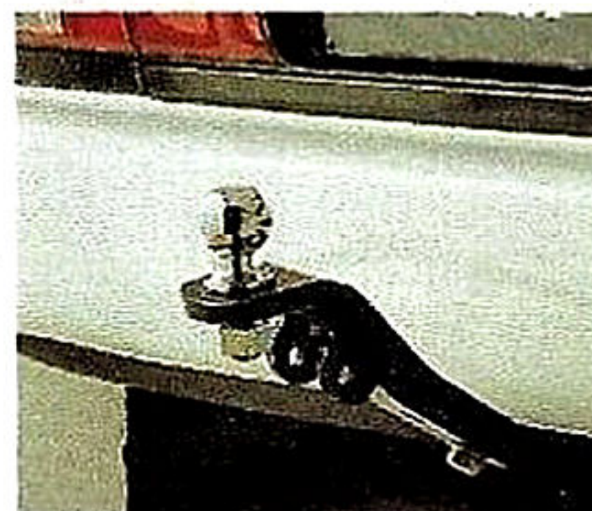
Tow bar with wiring harness, tongue and chrome ball.
