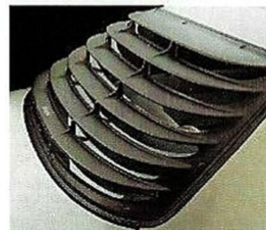
Rear louvre shades assist in lowering cabin temperature.
