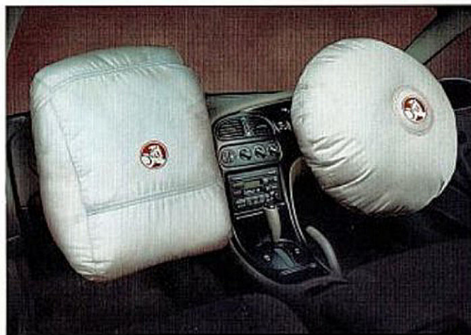
Driver and front passenger airbags The Commodore Acclaim features a driver and front passenger airbag system as standard equipment. These deploy simultaneously in milliseconds in conjunction with Commodore's front seat belt pre-tensioners. They also use 'wheeler' technology to prevent aggressive airbag injuries.
