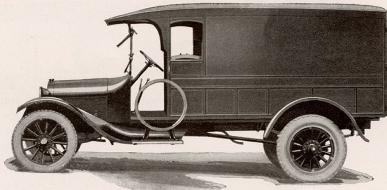
Truck Chassis with No. 2085 Full Panel Body. Furnished in 1-ton and 1½-ton capacities. Loading space 108" long, 51" wide, 58" high
