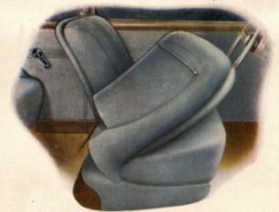
For Easy Access to the rear seat of all two-door types, each front seat back tilts inward, away from the wide door, as it swings forward. Every detail of the Mercury has been considered in the light of comfort and convenience.
