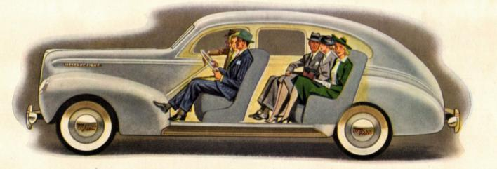
Center-Poise Design cradles passengers between springs that are more than 10½ feet apart. The compact V-type engine permits more usable length inside the body. You ride insulated from bumps by Triple-Cushioned Comfort: Soft-edged seat cushions with deep inner springs; large, double-acting hydraulic shock absorbers; long, flexible springs.
