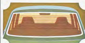
ELECTRIC REAR WINDOW DEFOGGER. ALL 1600 MODELS.
