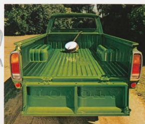
The 7 ft., 2 in. cargo bed is a full 15.9 inches longer than on the standard bed.
