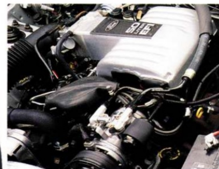
The 5.0 liter V-8 has individual port electronic fuel injection, an aluminum intake manifold and individual runners.
