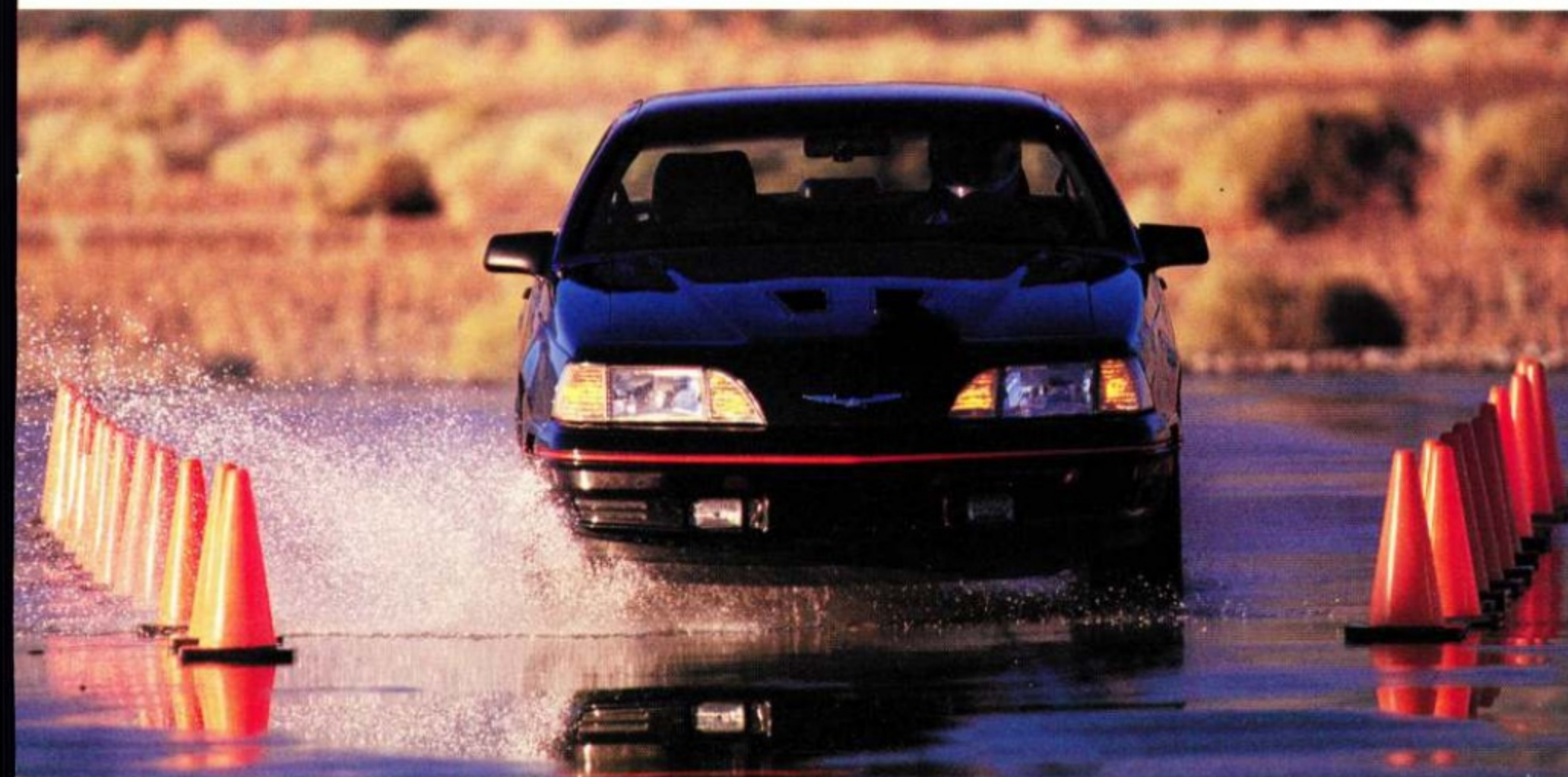
Turbo Coupe's anti-lock system "pumps the brakes" rapidly and repeatedly, allowing the driver to maintain control under many circumstances that would normally mean a skid.
