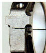
Connecting rod bearing caps are mechanically fractured so they can be reassembled only one way: precisely.
