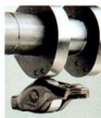
Roller finger cam followers are but one of many friction-reducing features in this advanced V-8.
