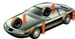
At 55 mph, Mark VIII's computer-managed suspension actually lowers the automobile so that its riding closer to the road.
