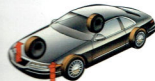
The SLA front suspension is designed with anti-dive geometry to counteract the automobile's tendency to "dive" when braking.
