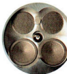
Each cylinder's combustion chamber breathes in and out freely through four valves.
