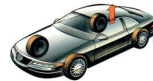
Air springs maintain the proper ride height and a smooth ride regardless of vehicle loading.
