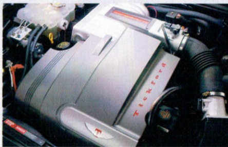
The TS50's 220kW Synergy 5000 V8 engine.
