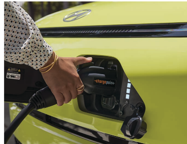
Standard 400V DC Fast Charging with state of charge light
