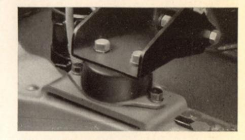
The Cadillac V-8 engine is firmly mounted and insulated from the frame by three rubber cushions.
