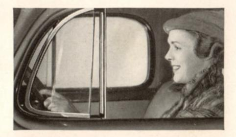
Adjustable Fisher No-Draft Ventilation circulates fresh air in any weather, free from disturbing drafts.
