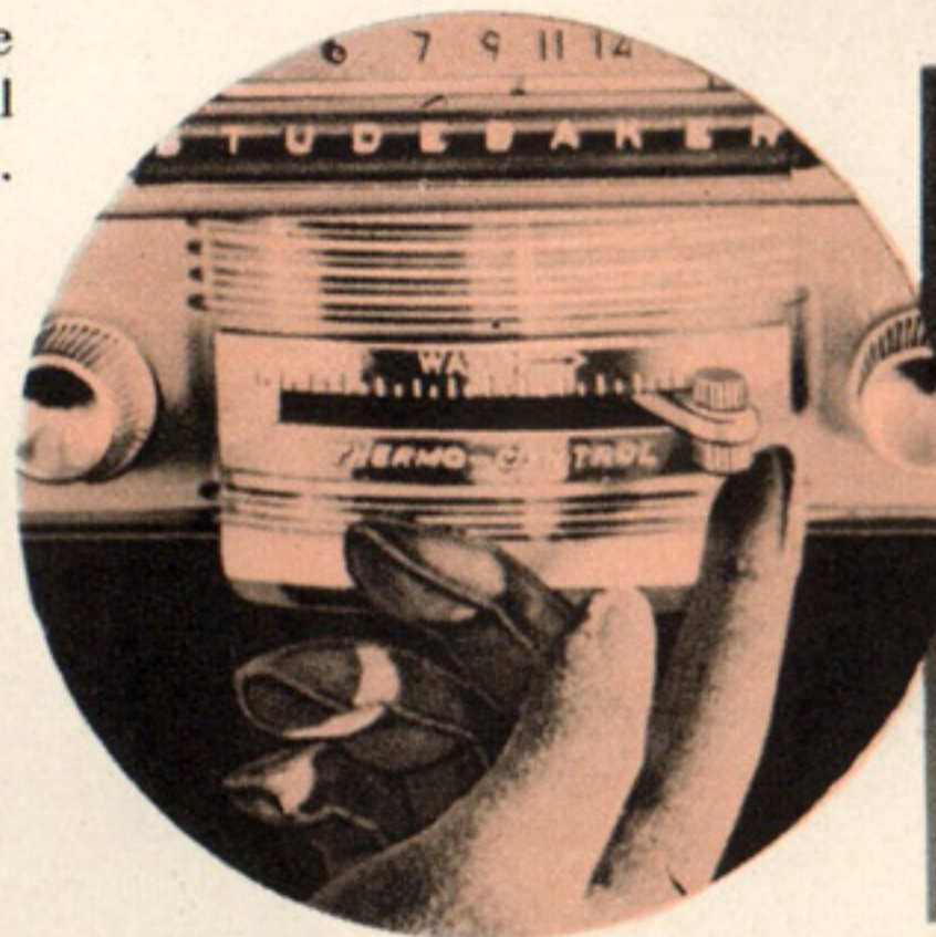
New Climatizer "Thermo-Control" permits accurate regulation of heat flow. Move to right to increase heat, to left to decrease or shut off heat. Knobs regulate defroster and flow of fresh ventilating air.
