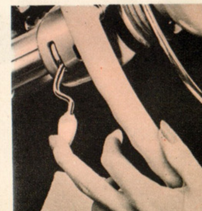
Built-in Directional Signaling Equipment provides convenient lever at your finger tips on left side of steering column with which to signal turns to following and approaching traffic. Special bulbs in fender and tail lamps flash brilliant warning signal. Signal turns off automatically.
