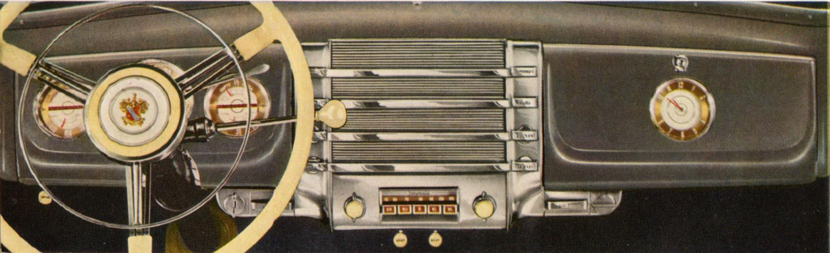
The handsome instrument panel of the SPECIAL puts the driving instruments right in the driver's line of vision. Lights, heater and accessories are controlled by switches that form extensions of the bars of the radio grill. To the right are the clock and fresh-air adjustment.
