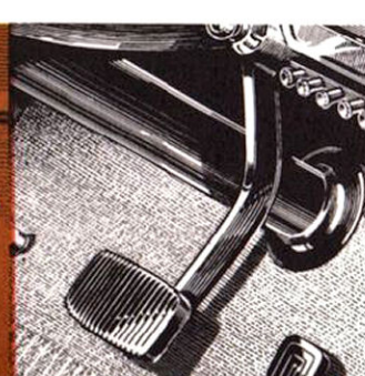
Pendant-type Pedals eliminate openings in the floor boards—reduce road noise and dust.
