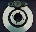
Big, powerful 10.75-inch disc brakes up front assure you the stopping power worthy of a GT built by MG.
