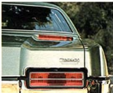
Two sets of tail lights. Toronado's distinctive styling includes a second, eye-level pair of tail lights for increased visibility.
