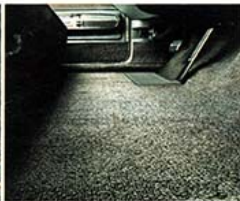
A completely flat floor. Toronado's front drive eliminates that hump inside—gives you more legroom, front and back.
