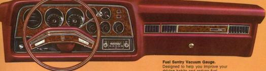
driving habits and reduce fuel consumption. Gauge needle alerts you when low engine vacuum is robbing fuel, indicates when gas mileage is "good" or "poor." Fuel Monitor Warning Light is also available. Uses light instead of gauge.
