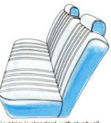
vinyl trim is standard, with sturdy allvinyl trim available as an option. LTD II Series feature flight bench seat with a fold down center armrest and bucket seats as an option. (LTD II Series flight bench and bucket seats are standard construction without heavy-duty components.)
