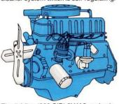
The 5.0 litre (302 CID) 2V V-8 engine is another partner for law-enforcement vehicles. Its features include hydraulic valve lifters, high-turbulence combustion chambers for clean-burning combustion, and slipper-type pistons to help eliminate scuffing of cylinder walls.
