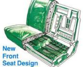
LTD's new front seat design provides good driver comfort for all-day patrol duty. The molded-foam back padding is mounted directly to the steel seat-back, without intervening springs, thereby reducing overall thickness and helping
