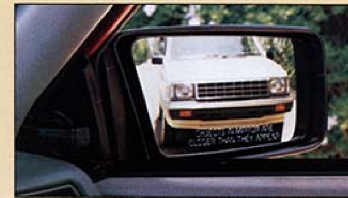
Deluxe and XE models come with a standard convex passenger side mirror, remotely controlled from inside.
