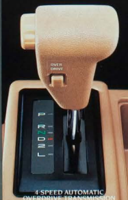
4-SPEED AUTOMATIC OVERDRIVE TRANSMISSION
