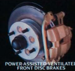
POWER-ASSISTED VENTILATED FRONT DISC BRAKES
