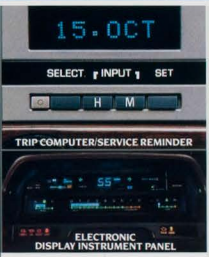
INSTRUMENTATION Electronic Display has speedometer and automatic transmission indicator. Trip Computer/Service Reminder checks engine operation.
