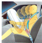
Height adjustable front seat belts, with belt lockers to minimise payout of seat belt webbing in extreme conditions.
